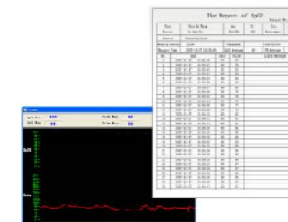
Provides up to 100 IDs and 300 hours data storage capacity for continuous monitoring. All data can be transferred to PC through DB9 interface for storage, review and printing.
